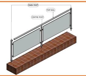
Made 2 Measure Factory Assembled No Welding Glass Balustrade
